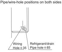
Pipe/wire-hole position on back side
