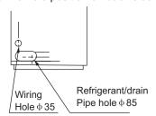
Pipe/wire-hole position on the bottom
